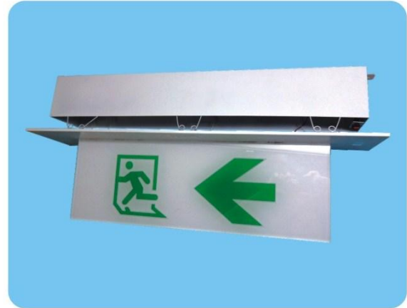
JXP8SNH2-Elite-F, 1x8W emergency sign white escape route sign with left directional arrow on green, c/w NI-MH rechargeable battery.
